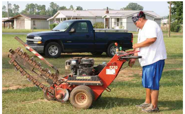
Nick Behan unloads the trencher that will be used to dig ditches for electrical lines
